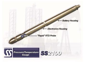
tions. As seen in the graph below, the external RTD has a response time ten times faster than the internal temperature sensor found on most gauges. This is primarily due to the amount of mass surrounding the internal sensor.
